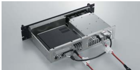
IC-FR5100H series has built-in power amplifier unit.
